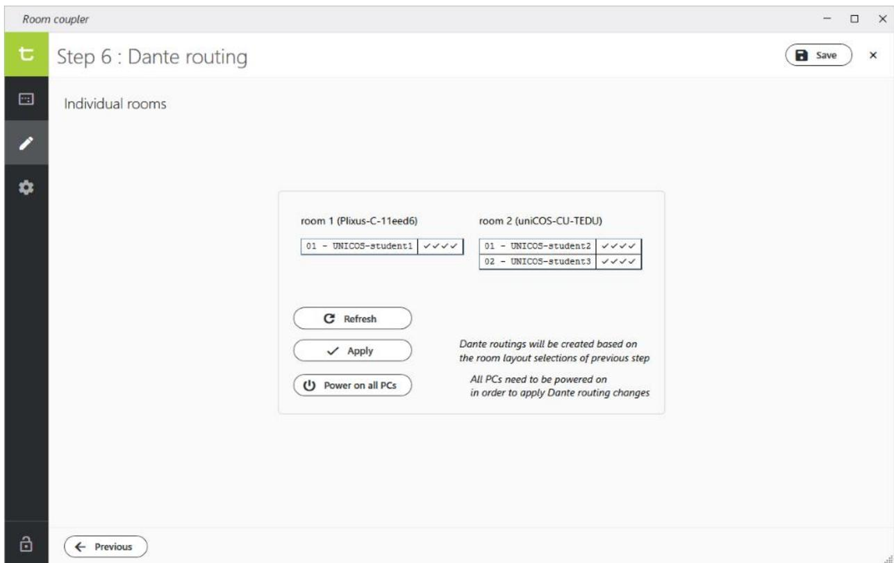
The lists in the screenshot above show all booth PCs in each of the rooms (only 3 PCs in total for this small test setup). The 4 checkmarks next to each PC show that all 4 Dante routings are correct for the PC (there is a 2-channel audio stream in each direction, resulting in a total of 4 streams per PC).
