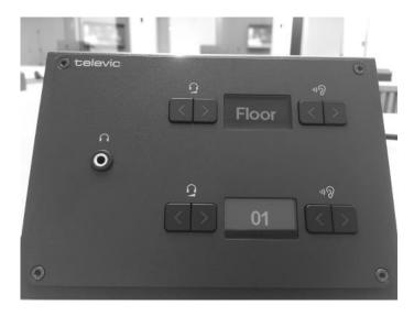
A Televic interpreter training system is typically equipped with "dual channel" listening panels. This allows you to **listen to source and translation simultaneously**. Select the "Floor" signal on the topmost selector in order to hear the speech in your left ear. Select a booth on the lower selector in order to hear the translation from that booth in your right ear. The volume for each of both signals can be adjusted separately.
